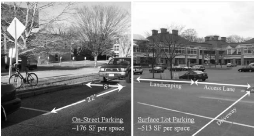
Fig. 2. Land Use of On-Street Parking versus Off-Street Surface Lot. Source: W. E. Marshall.
